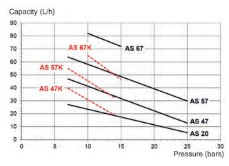
Data shown take into account a wear margin. Do not oversize the pump when selecting the gear capacity.
